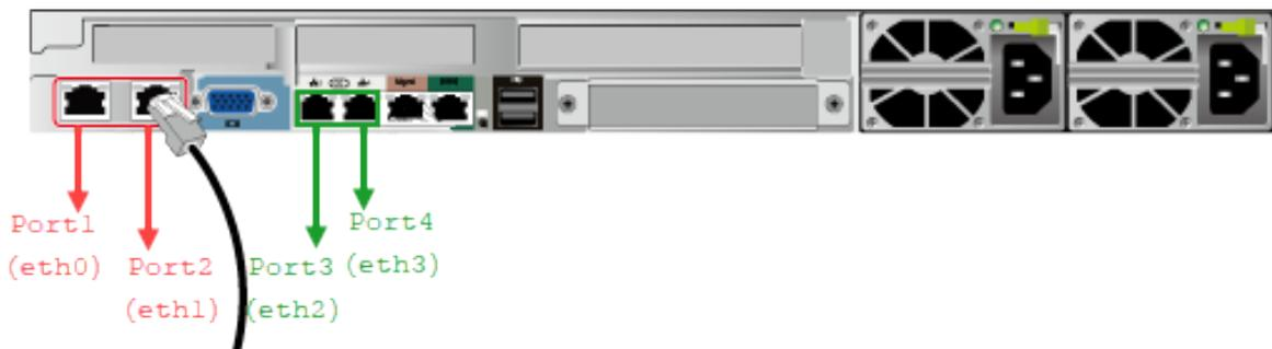
The default names of network interface card (NIC) recognized by Yeastar S1000-P IPPBX are eth0 and eth1. It means you can connect a network cable to Port 1(eth0) or Port2(eth1) directly to access the network.
